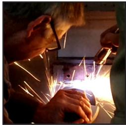
2. Grind/cut and sand welds to remove existing spacer plate and restore original smooth door surface
