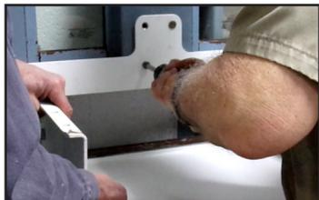
5. Locate, align and install 4 bolts using existing 3/8-16 threads
