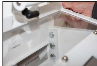
10. Insert 8 each carriage bolts (4 each side) and tighten acorn nuts with 5/8" socket using care not to overtighten.
