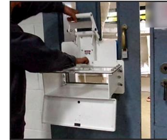
12. Operate outer door 1) Disengage slam latch from catch plate by pulling down, allowing door to swing open. 2) To close, swing door up to engage slam latch, into catch plate
