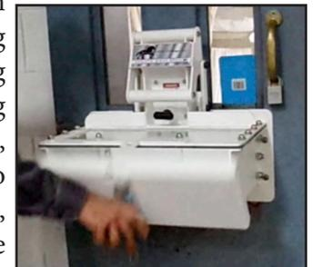
13. Operate Pepper Spray Port 1) Open inner door just enough to insert hose. 2) Unscrew cap, insert nozzle, spray. 3) Replace port cap when finished.
