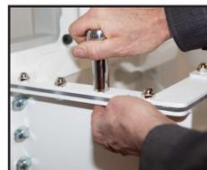
11. Operate inner door 1) Pull and hold T-handle on spring pin, 2) Grasp and raise inner door handle to fully upright position, 3) Release T-handle allowing spring pin to secure inner door in the upright open position.
